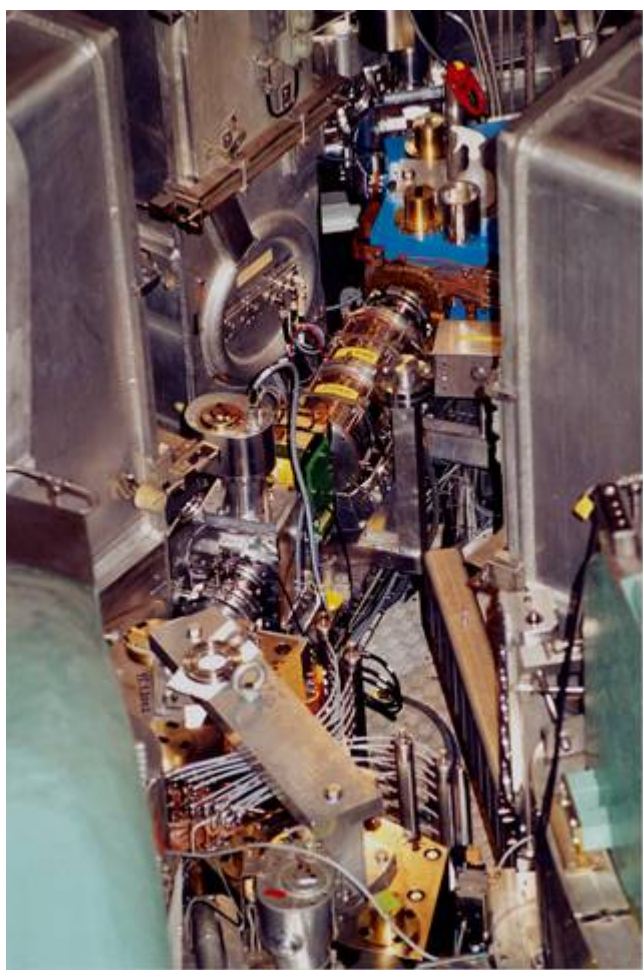
Fig. 2: Beam line section in the ring centre. The beam enters in front of the magnet at the top and leaves via the two magnets at the bottom.
