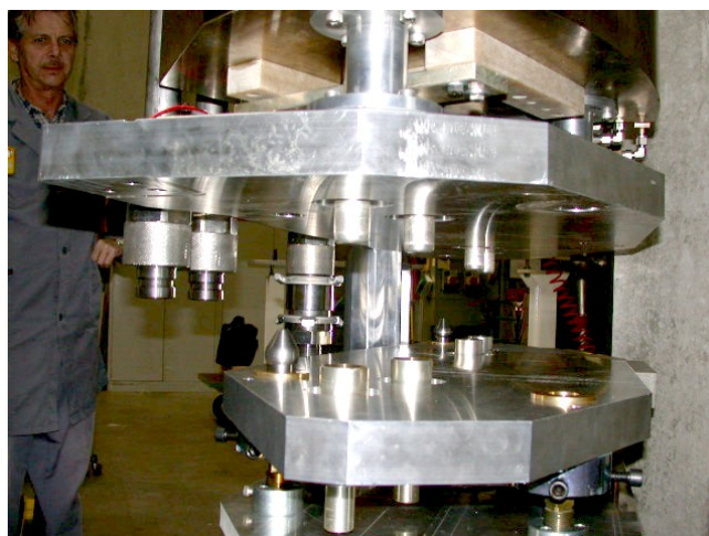
Fig. 7: The AND module in the connection plane. The electrical and water supply connectors as well as the positioning pins can be seen. The upper plate with the electrical contact pins and positioning holes and slots is the module base plate. The lower plate, with the receptacles for the electrical connectors and the mechanical positioning pins, is fixed. A duplicate serves as parking plate when the magnets must be removed from the centre for repair under reduced radiation exposure conditions or for preparation and pre-adjustment of the replacement magnets.
