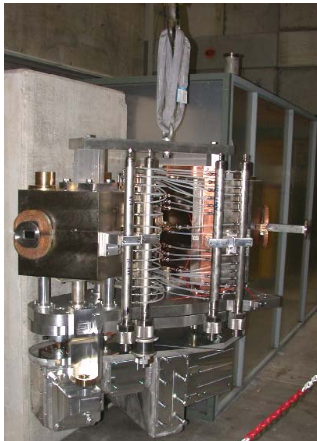
Fig. 12: The AND module during test assembly. One of the water supply manifolds is fitted with a quick coupler. The crane is attached at one point above the centre of gravity of the module. The main guide pin (front left) is not yet mounted.
