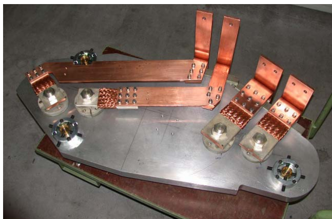
Fig. 6: The underside of the AND fixed plate showing the electrical connections from the flexibly mounted receptacles to the lugs where the supply cables will be attached, together with the supporting adjustable feet.
