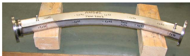
Fig. 11: The AND02 vacuum chamber with its welded positioning pins. The integrated bellows (left) enables the connection to the AND01 vacuum chamber to be made in a minimum of space using a standard chain fastener together with an aluminium seal.
