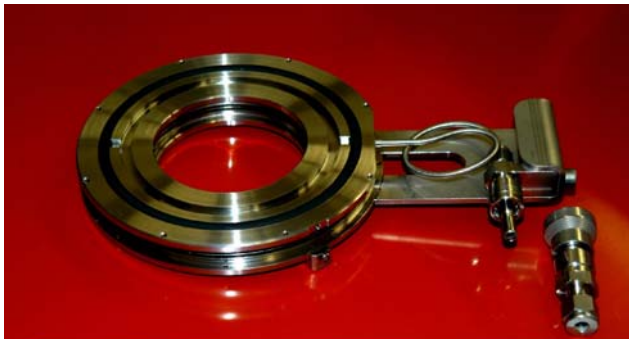
Fig. 9: The expandable vacuum connector together with its compressed air quick coupler ready for use.
