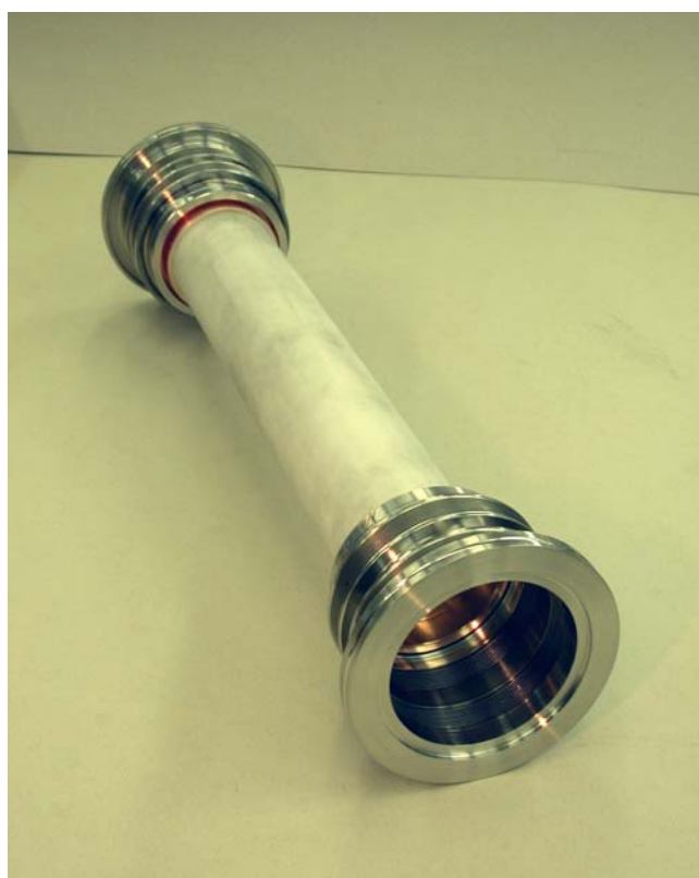
Fig. 1: UCN vacuum chamber with integrated bellows.
