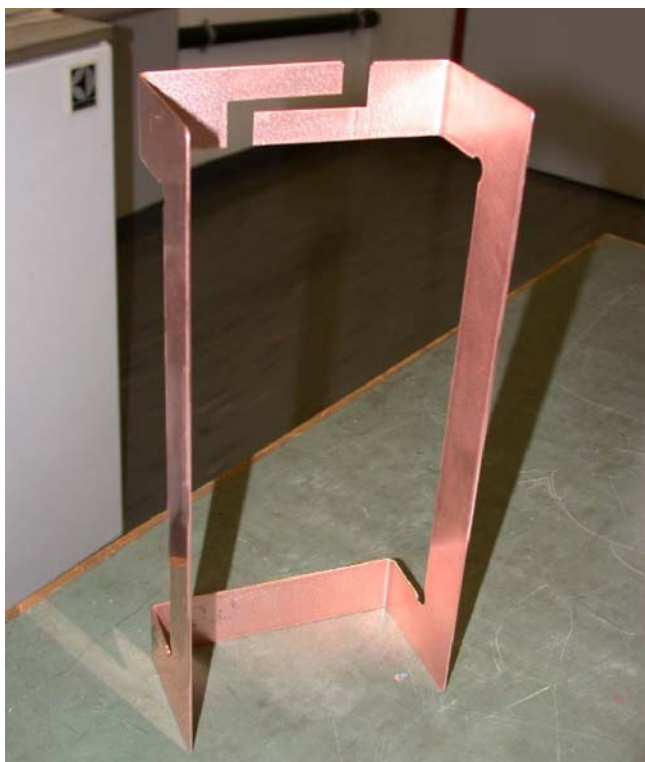
Fig. 2: One of the 18 different turns ready for insulating.
