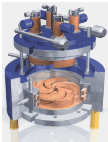
Fig. 2: Artist view of the superconducting cyclotron COMET (courtesy of ACCEL GmbH). The accelerator will be optimised for a stable well-controlled intensity of the beam and for high extraction rates.
