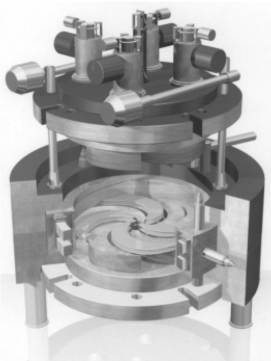
Fig. 1: COMET: C ompact M edical T herapy C yclotron. The pole cap is lifted for access; the four dees, the magnet hills and the two superconducting coils with their cryogenic helium vessel can be seen. (By courtesy of ACCEL).
