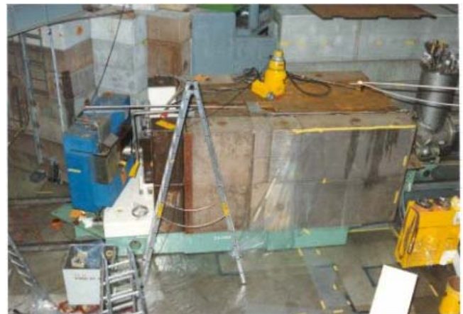
Fig. 1: The photo shows the old insertion wagon with its shielding made of iron-concrete. On the left, the first bending magnet ASK61 is visible. This magnet will be replaced by a magnet with radiation hard coils because of its exposure to target E. On the right, it is possible to recognise a part of the superconducting \mu -channel. The \mu E4 wagon will be reused for the new components.
