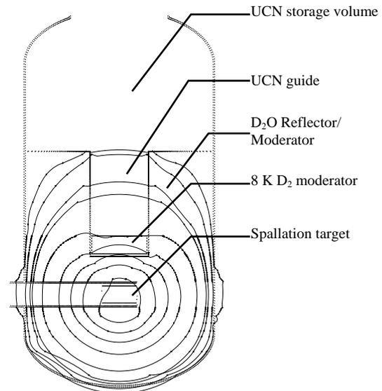
**Fig. 1:** Neutron flux contours superimposed onto an outline of the SUNS source. Contours are shown for flux levels of 10, 8, 6, 4, 2, 1, 0.8, 0.4 and  $0.2 \times 10^{13}/\text{cm}^2/\text{sec}$  for 1 mA proton current are shown.
