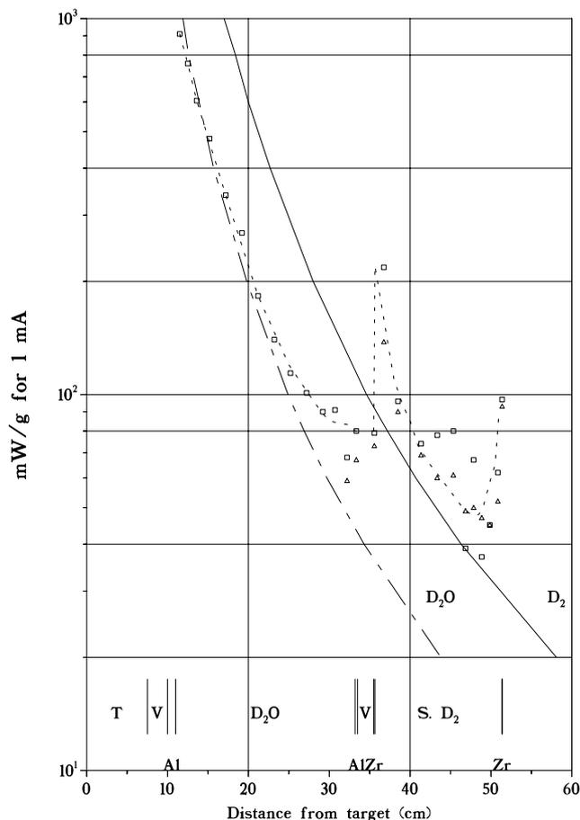
**Fig. 3:** Calculated power densities along the vertical axis of the SUNS system (dashed line with squares and triangles). The other two lines are the results from the PNPI calculation (solid for the D<sub>2</sub> and double-dashed for the D<sub>2</sub>O). The actual media in the various regions are indicated by the symbols along the bottom (T = target, V = vacuum).
