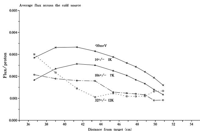
**Fig. 2:** Variation of the neutron flux across the cold moderator modelled as 8K D<sub>2</sub> gas. The four curves shown are the contributions of the three Maxwell functions and the total intensity below 10 meV.
