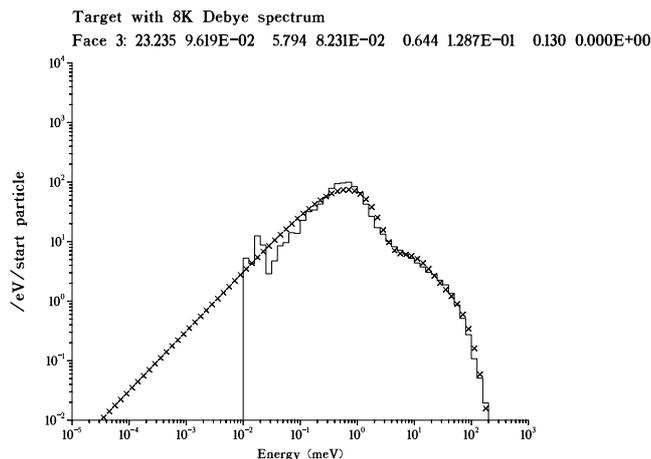
**Fig. 4:** The spectrum of neutrons escaping the upper open face of the moderator (histogram) with the result from fitting the data to the sum of three Maxwell flux spectra (shown by crosses). The target Deuterons in the scattering have a Debye spectrum at a temperature of 8 K.
