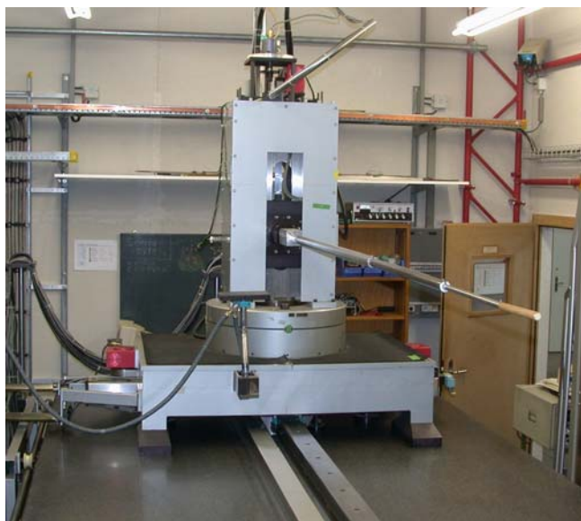
Fig. 1: Magnetic field measuring machine with the measuring arm that supports a Hall probe covered with a protective insulating cap.
