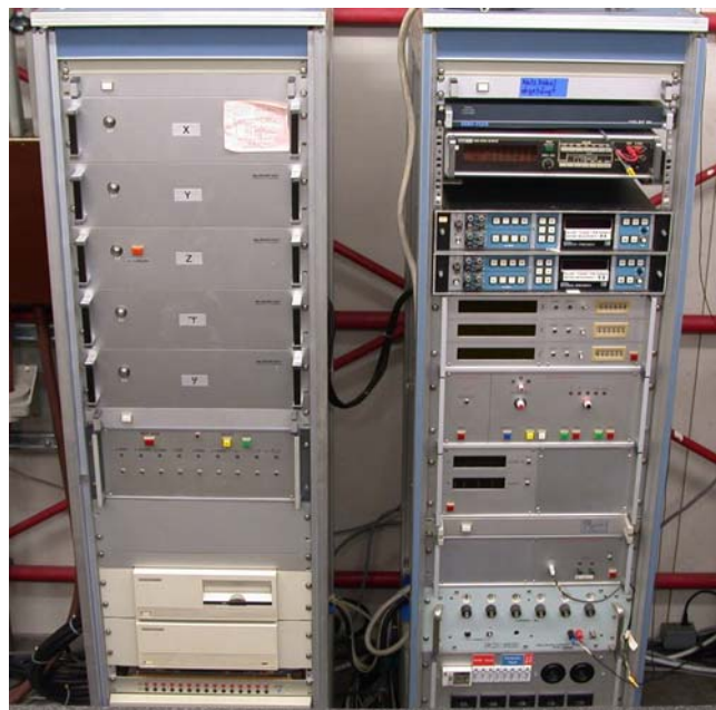
Fig. 2: The old HP 1000 A-900 computer with two DATA PRECISION 7500 digital multimeters and the electronics for controlling measuring machine position.
