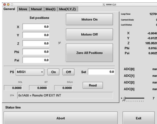
Fig. 4: Graphical interface of the new program for controlling the machine position, setting the magnet current and measuring magnetic fields in time or in space.
