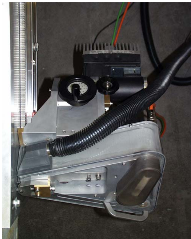
Fig. 3: Bottom view of polishing module as it swings around the end of the beam slit. Shown is the belt and its fixture, and the dust pick-up hose leading to the vacuum cleaner.
