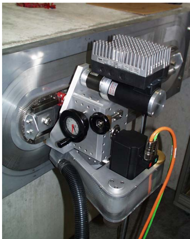
Fig. 2: Grinder/polisher module on support plate, installed on dummy cavity gap.
