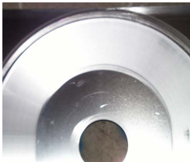
Fig. 4: Final result of a successful grinding and polishing process; shown is one end of the 'racetrack'-shaped sealing surface around the end section of the beam slit.
