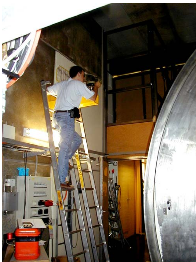
Fig. 4: Measurement of the height of the object reference marks on top of the Gantry 1, using our WILD N3 precision level instrument.
