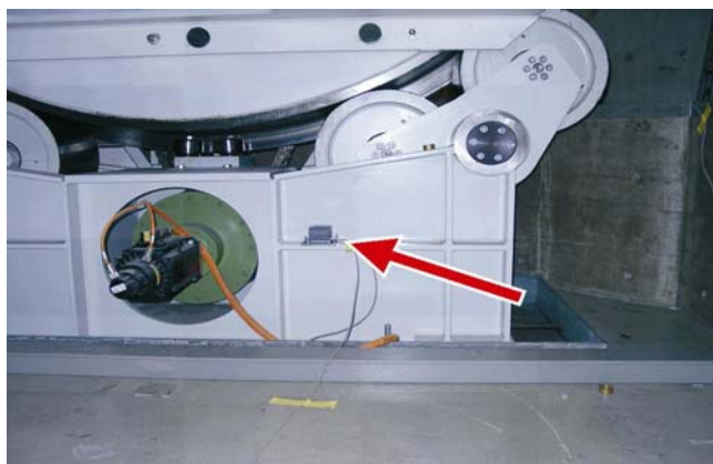
Fig. 1: The picture shows the support frame of Gantry 1. The arrow indicates the location of the inclination sensor N2.
