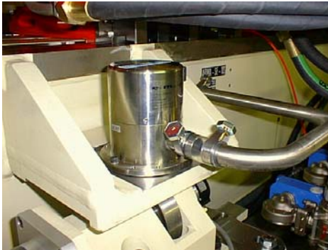
Fig. 1: HLS-Level sensor mounted on a girder.
