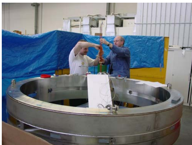
Fig. 3: Assembly of the magnet cryostat (Photo by courtesy of ACCEL).
