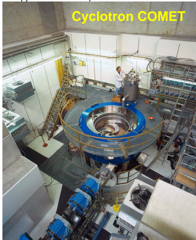
Fig. 2: shows the mounting of the superconducting cyclotron COMET from ACCEL Instruments GmbH in May 2004. The accelerator is housed in a bunker with 3 to 4 m shielding walls. Visible in the foreground are beam extraction area and first part of the beam line.
