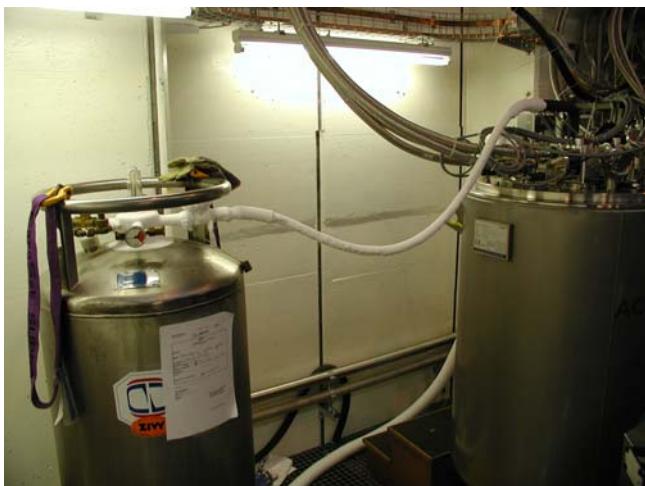
Fig. 4: Cooling down using liquid nitrogen.
