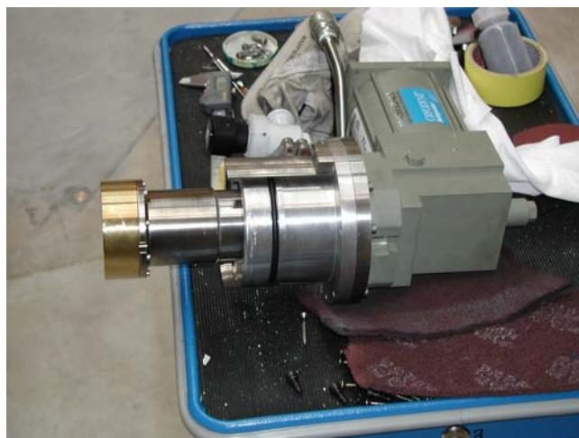
Fig. 3: One of two single stage Gifford-McMahon shield cooler cold heads (Helix CTI).
