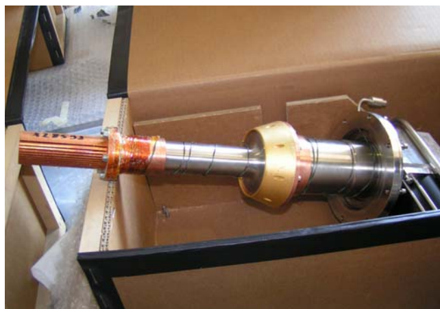
Fig. 2: One of four reliquifier two-stage Gifford-McMahon cold heads (SHI Sumitomo Heavy Industries).
