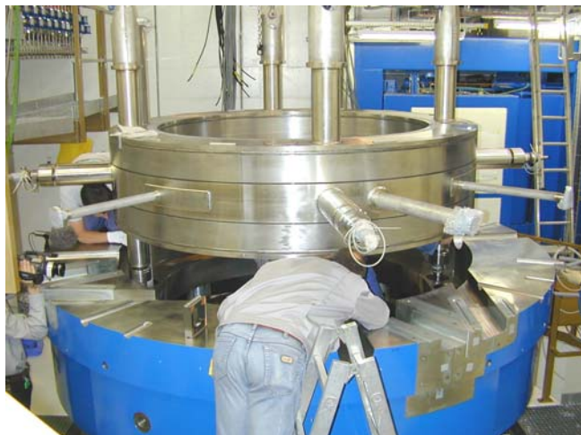
Fig. 1: Mounting of the coil cryostat in the iron yoke at PSI.
