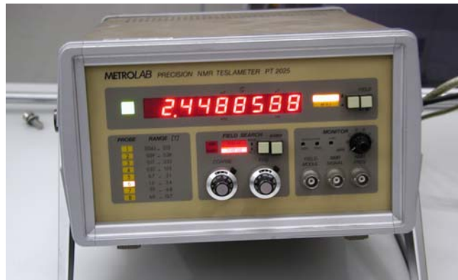
Fig. 5: NMR measurement of the magnetic field in the centre of the cyclotron at the first powering at PSI.
