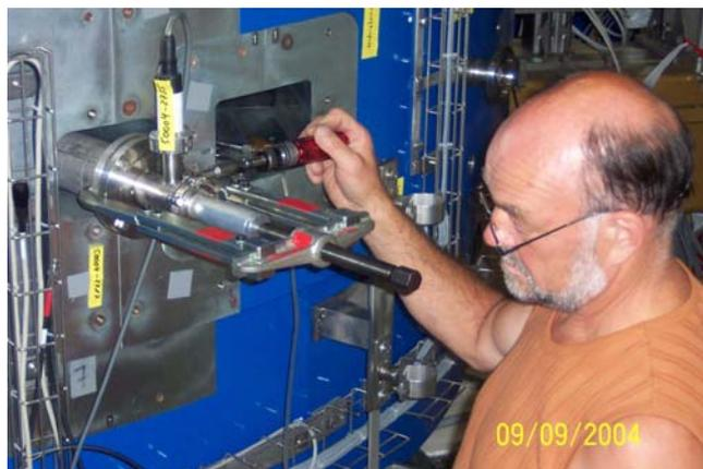
**Fig. 4:** In-situ exchange of chain clamp KF 40.
