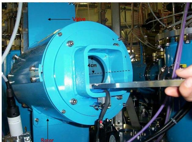
**Fig. 2:** Shielding of magnet fields for the operation of the turbomolecular pumps.
