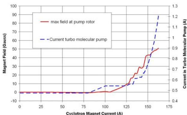
**Fig. 3:** The measured magnetic field inside the shielding at the rotor position and the pump current vs. current in the superconducting coils of the cyclotron magnet.
