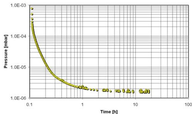
**Fig. 1:** The pump down curve, recorded on Nov 19<sup>th</sup>, 2004, shows that all requirements for the vacuum system have been achieved.
