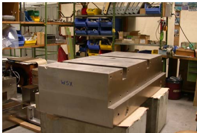
Fig. 2: The WSX solenoid base plate weighing 4.7 tons. The WSX forms part of the new \mu E4 beam line (LEM beam line). The plate did not have to be machined for the thickness of 450 mm.
