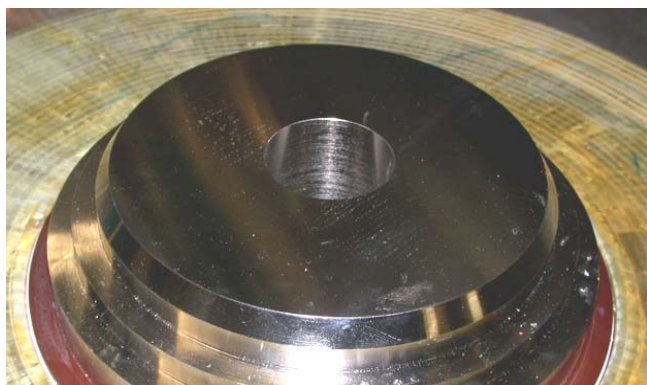
Fig. 6: The exposed pole of the BBC magnet after drilling.
