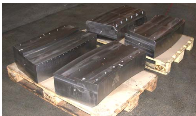
Fig. 5: Four yokes for two spare AHA magnets. Together, they weigh about 2.3 tons. This magnet is the 590 MeV Ring extraction magnet, which operates within the vacuum chamber of the cyclotron and is exposed to radiation due to the extraction losses. Maintenance is therefore difficult and it is imperative to have spares ready for operation. This work is performed by our colleagues from ABE.
