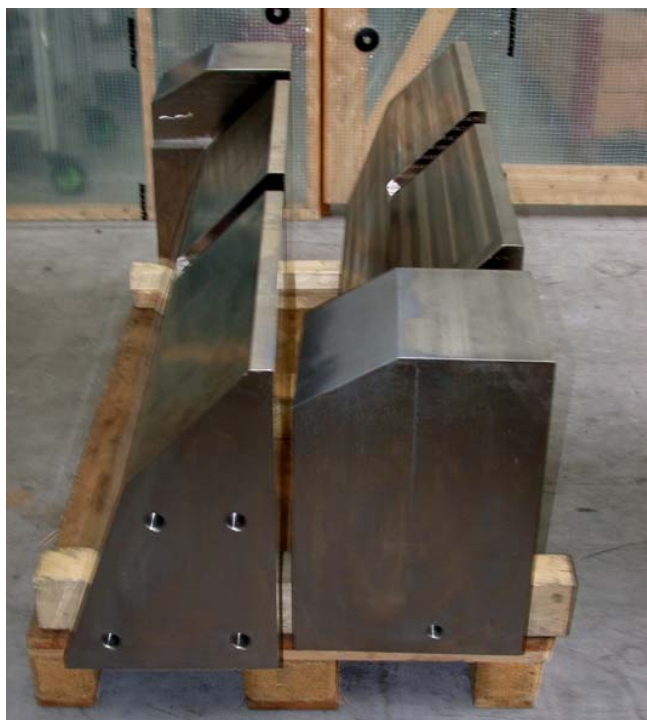
Fig. 4: The WSX solenoid upper return yokes each weighing 1.22 tons.
