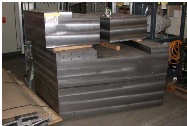
Fig. 3: The two larger lower pieces will form the magnet yoke for a spare AHC magnet. The blocks on top are for a spare AHB magnet. AHB weighs about 4 tons and AHC 15 tons.
