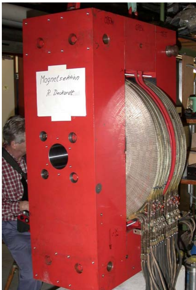
Fig. 8: The modified 5 ton BBC magnet after drilling the central large hole, four new bolt holes and a ring of threaded holes to attach the experimental vacuum chamber. This work was performed at PSI in the main workshop.
