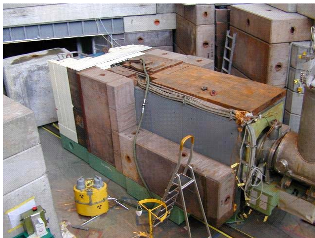
Fig. 1: The old insertion wagon with its rusty shielding after extraction in January 2004.
