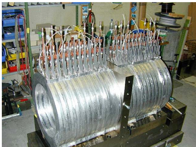
Fig. 3: The WSX solenoid with its coils from Novosibirsk during assembly. Each coil pancake consists of electrical windings on both sides and cooling plates in the centre. To keep the conductors and cooling components in position and to guarantee a good heat flow, they are cast in soft solder under vacuum.
