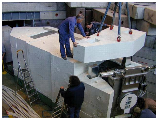
Fig. 2: The insertion wagon with its new beam line components packed in 100 tons of white painted cast iron shielding. The vacuum system can be partitioned with a slide valve, visible in the bottom right hand corner.
