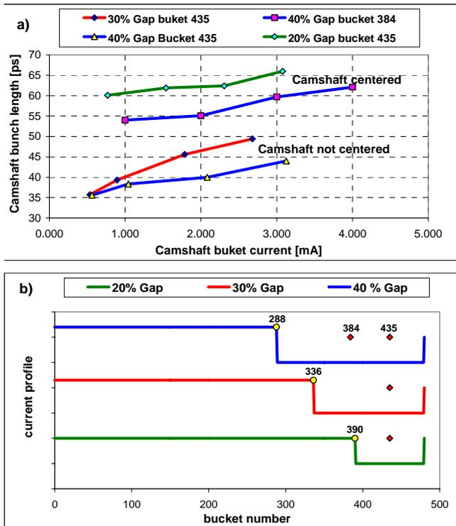
**Fig. 3:** (top) length of the camshaft bucket for different filling pattern configurations, (bottom) filling pattern profiles (continuous line) and location of the camshaft buckets (diamonds) during the streak camera measurements.
