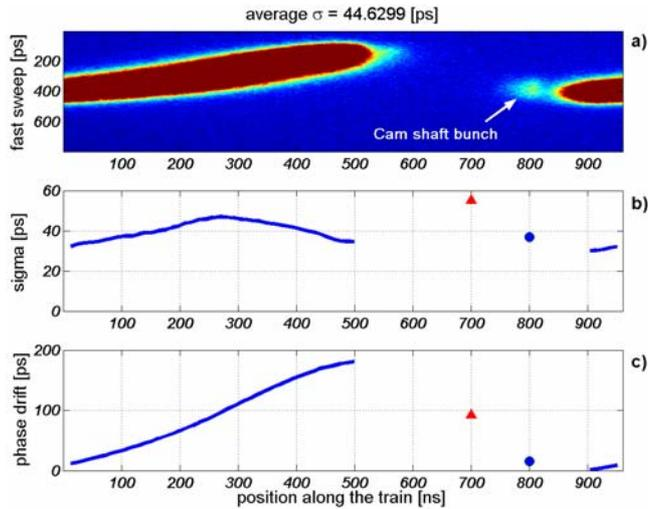
**Fig. 2:** **a)** Streak camera snap shot with 40 % gap in the filling pattern and a camshaft bucket at 90 ns from the train tail. **b)**  $1\sigma$  bunch length along the train and for a centered (triangle) and non-centered (circle) camshaft bucket. **c)** Phase drift with respect to synchronous phase. The camshaft bucket in the middle of the gap (at “zero” phase crossing) experiences the largest lengthening.
