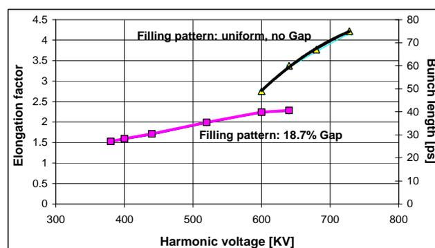
**Fig. 1:** Streak camera measurement, average bunch length in the SLS storage ring with 300 mA uniform filling pattern and with 18.7 % empty gap.
