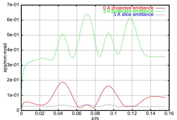
**Fig. 6:** Evolution of emittance (projected for zero current and 3 A and projected for 3 A) in the gun.
