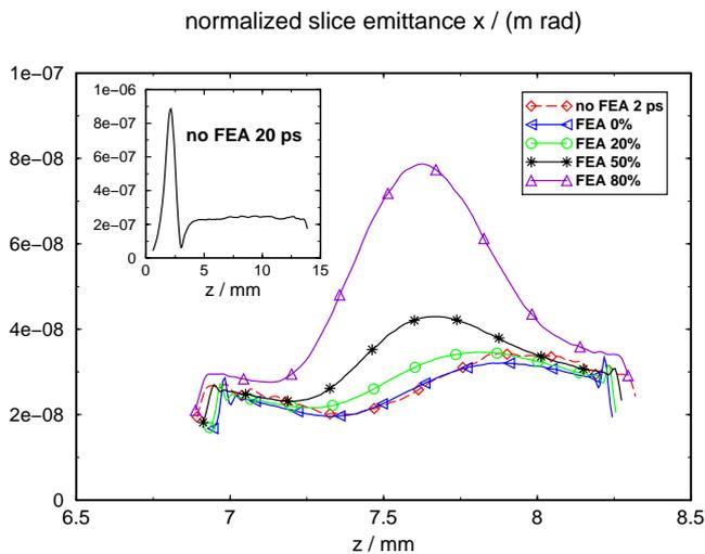
**Fig. 8:** Normalized slice emittances of the 2 ps FWHM bunches. “no FEA” refers to a smooth initial current distribution, whereas “FEA x%” denotes an emission from a FEA with x percent single emitter uncorrelated failure probability. Comparison with the slice emittance of a 20 ps FWHM bunch shows the influence of wake fields. All slice emittances have been calculated using a Gaussian weighting function with a sigma of  $1/100$  of the bunch length (about  $13\mu\text{m}$  for the 2 ps cases).
