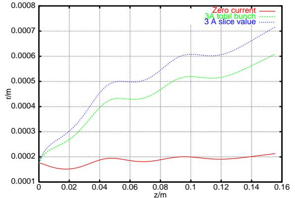
**Fig. 5:** Rms beam radius inside the gun for various currents.
