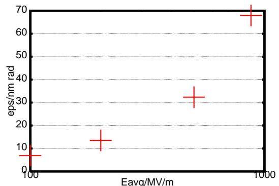
Fig. 2: Emittance due to nonlinear transverse fields in the iris at near zero current ( $I=1\mu A$ ).
