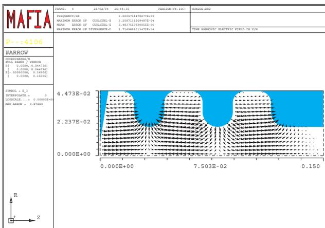
**Fig. 4:** Accelerating field in CTF gun 4.
