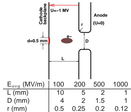
Fig. 1: Basic diode structure
