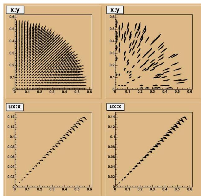
**Fig. 7:** Effect on transversal particle distribution and phase space for FEA simulations with 0% and 80% failure probability, at  $z = 9 \text{ mm}$ . Positions are indicated in mm.
