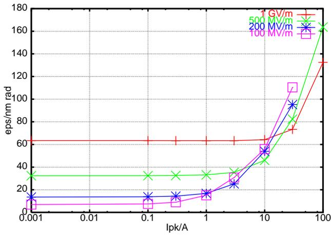
**Fig. 3:** Sliced emittance for the different designs and peak currents
