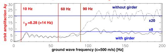
Vertical **orbit** PSD (1-60 Hz) without and with orbit feedback @ BPM ( $\beta_y$ =18 m):
