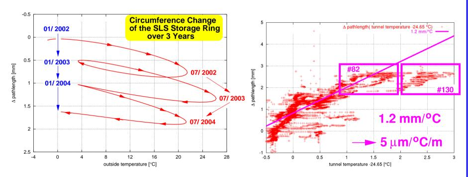
• Stabilization of the **tunnel temperature** to  $\approx \pm 0.1^{\circ}$  is needed to guarantee sub-micron movement!
