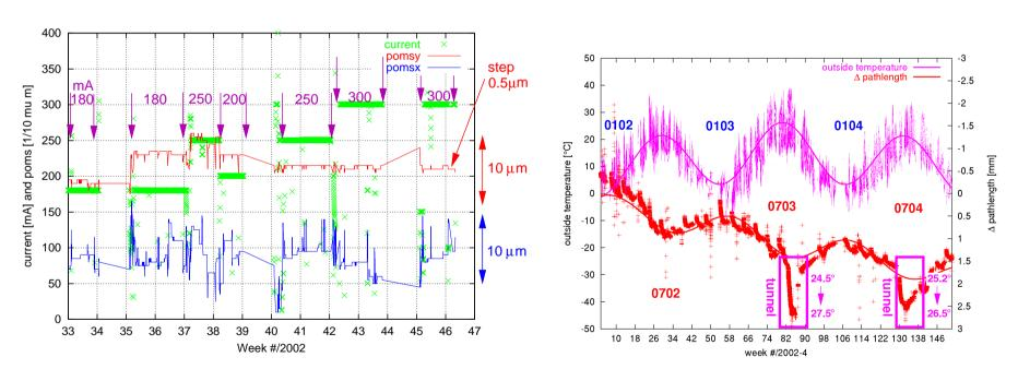
• Severe problems with the cooling capacity of the SLS during the hot summer 2003 (#82)! Again "scheduled" problems in 2004 (#130) due to the cooling system upgrade!
