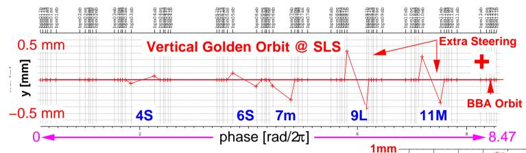
Golden Orbit: goes through centers of quadrupoles and sextupoles in order to minimize optics distortions leading to spurious vertical dispersion and betatron coupling (emittance coupling) + extra steering @ IDs
