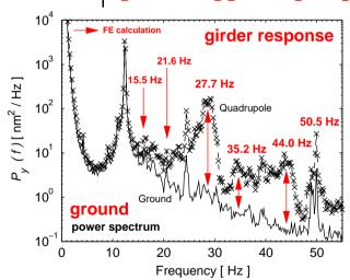
Vertical vibration PSD (1-55 Hz) measured on the slab and a girder (Redaelli et al.).
