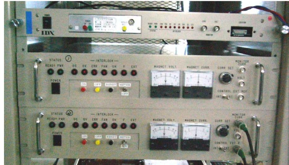
Power Supply Models for Fast Steering Magnets
