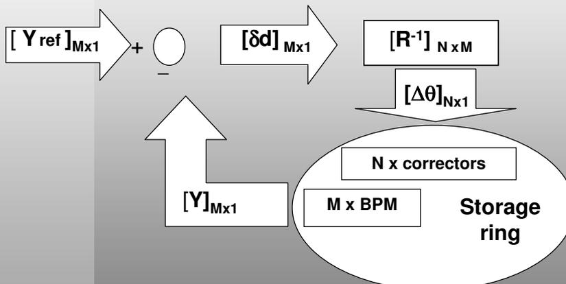
$$\text{Corrected orbit} = ([Y]_{M \times 1} - [Y_{ref}]_{M \times 1}) - R_{M \times N} \times [\Delta \theta]_{N \times 1}$$
