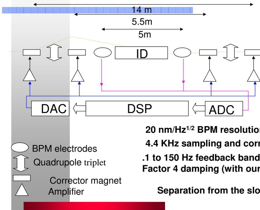
**20 nm/Hz<sup>1/2</sup> BPM resolution (1 μm in 2 KHz BW)**
