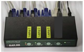
switch boxSwitchgreen LED = laptop readyred LED = laptop / document camera is connected to beamer
