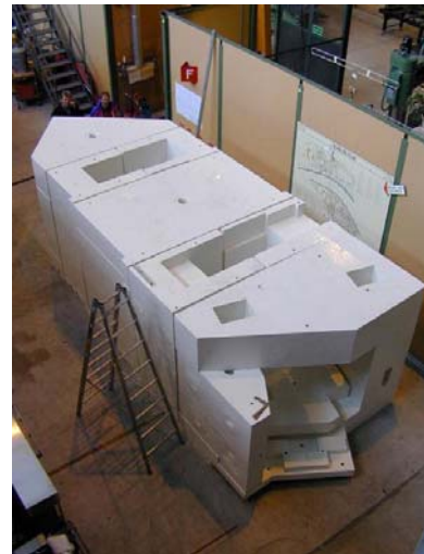
Fig. 2: The shielding of the insertion wagon which is made out of 22 cast iron blocks, with a total weight of 97 tons. The blocks are painted to allow decontamination and will replace more than 600 rusty iron bricks from the old superstructure.
