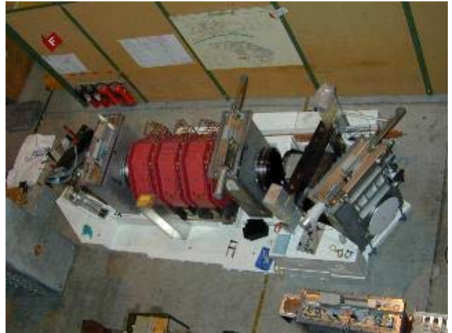
Fig. 1: The pre-assembly of the insertion wagon shows from left to right the first dipole, a slit, a quadrupole triplet and the second dipole magnet in between two beam blockers. Inside the second dipole there is a slit. The wagon sticks into the primary shielding.
