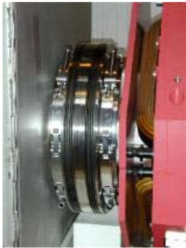
Fig. 3: A new vacuum chain connection system has been developed by the PSI vacuum section. It optimally applies the pressure to the seal and can be dismantled in a short time. The bellows can compensate geometrical errors and can provide space needed for replacement of components.
