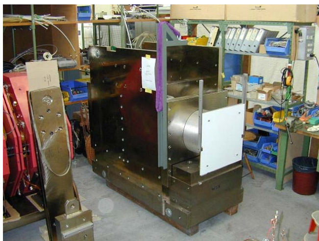
Fig. 6: This picture shows the mounting frame for the solenoid. For the first of three sections the lateral plates are removed, therefore one can see the vacuum tube. The inside of the vacuum tube is not visible because the end flanges of the beam pipe are covered as usual during mechanical work.
