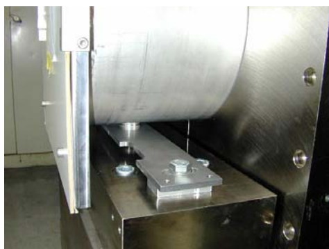
Fig. 7: This detail of the solenoid mounting frame shows the adjustment system for the vacuum chamber. A plate connected with the vacuum tube can be moved in the axial direction and fixed at the correct position with a large bolt. The adjustment must be done very carefully to avoid damage to the sealing surfaces.
