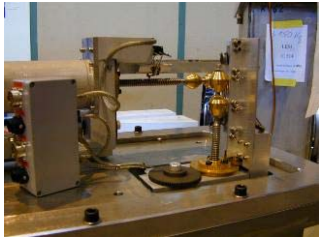
Fig. 4: This picture shows the drive unit of a slit system. We could redesign parts from existing slit systems. The drives are provided with excess-current switches and slipping clutches installed to prevent collisions. Unfortunately, it was not possible to relocate the drives of the horizontal jaws to more accessible positions.
