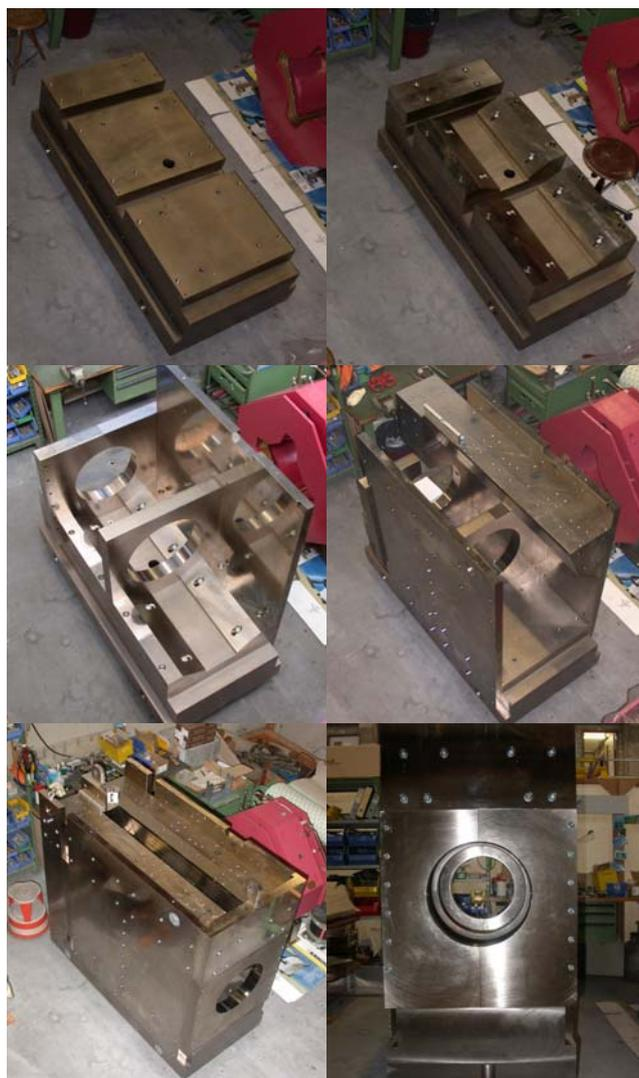
**Fig. 1:** Test assembly of the WSX iron yoke structure.
