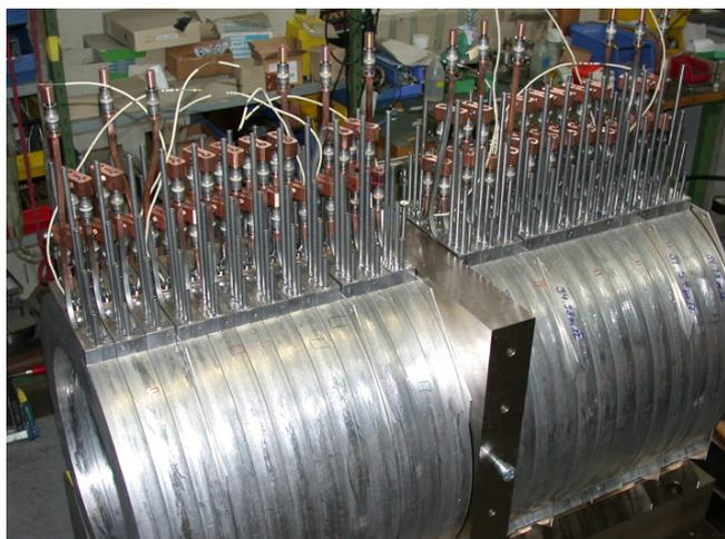
**Fig. 2:** Each of the two WSX solenoids is powered using 12 coils connected electrically in series.
