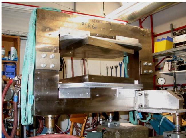
**Fig. 11:** ASR61 during the measurement process. The extended trapezoidal poles and the radiation hard coils can be seen. The two yoke pieces were made from the pole plates of a scrapped spectrometer magnet.
