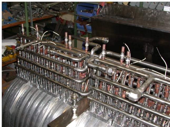
**Fig. 5:** The WSX stainless steel manifolds provide cooling water to all the coils in parallel. There are four independent water cooling circuits for redundancy.
