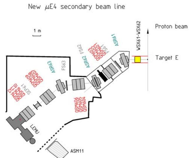
**Fig. 17:** Layout of the new  $\mu$ E4 beam line. LEMU is the attached experimental apparatus. ASM11 belongs to the neighbouring experimental area.
