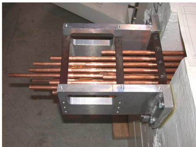
**Fig. 9:** The copper connection tubes for the first QSM triplet emerging from the end of the trolley.
