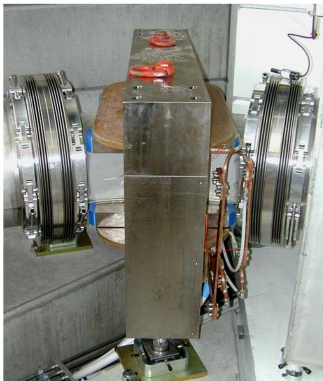
**Fig. 16:** The bending magnet ASR63 installed in the new  $\mu$ E4 beam line (LEM beam line).
