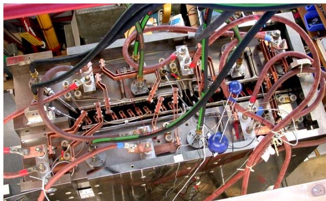
**Fig. 6:** The assembled WSX double solenoid with temporary power and cooling connections during the magnetic measurement and testing process.
