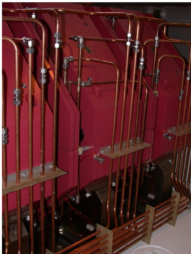
**Fig. 8:** The first QSM triplet installed on the trolley showing the copper cooling water and power supply tubes.
