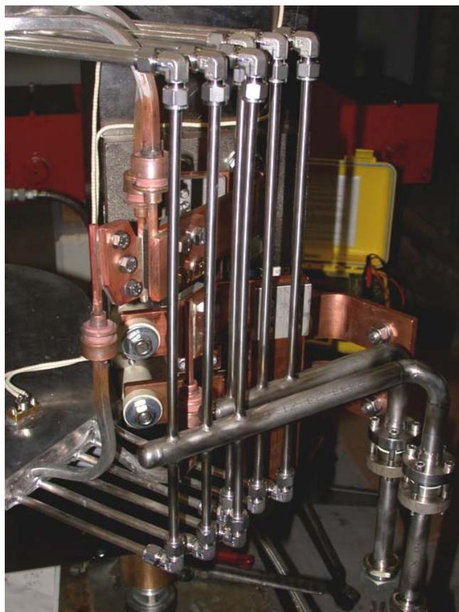
**Fig. 12:** The ASR61 electric and cooling connections, made in a very limited space. One can also see a thermoswitch with its connecting wires. They are insulated using hundreds of ceramic beads.
