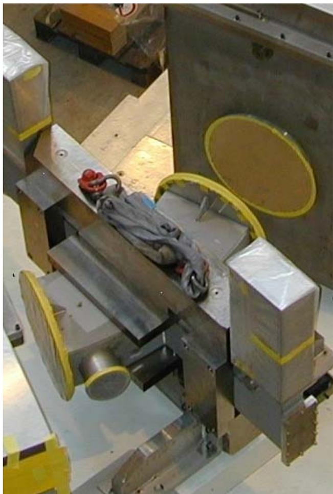
**Fig. 15:** The bending magnet ASR62 installed on the LEM trolley. The vacuum chamber side extensions for the movement mechanism of the integrated beam stopper passes through the side yokes of the magnet.
