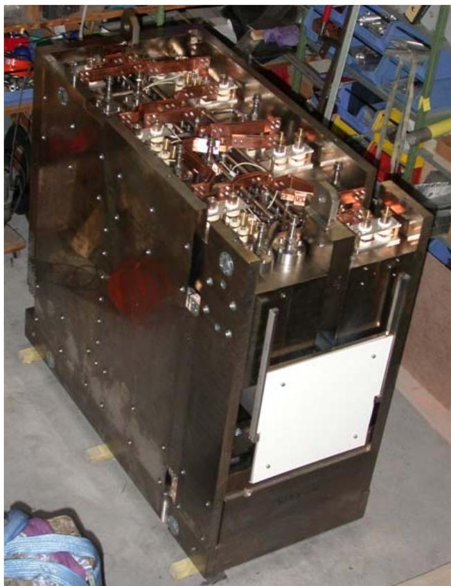
**Fig. 3:** The assembled WSX double solenoid with vacuum chamber. In operation, two parallel power supplies will be used for WSX61 and one for WSX62.
