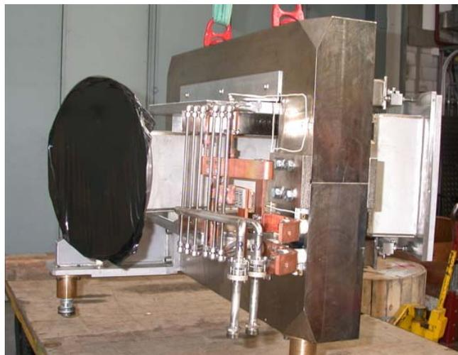
**Fig. 13:** The completed ASR61 with vacuum chamber ready for installation. All insulating components are made of ceramic due to the expected high radiation level.
