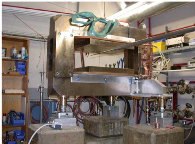
**Fig. 14:** ASR62 during the measurement process. The extended straight poles, the conventional glass-epoxy insulated coils and the holes for the special vacuum chamber in the side yokes can be seen.
