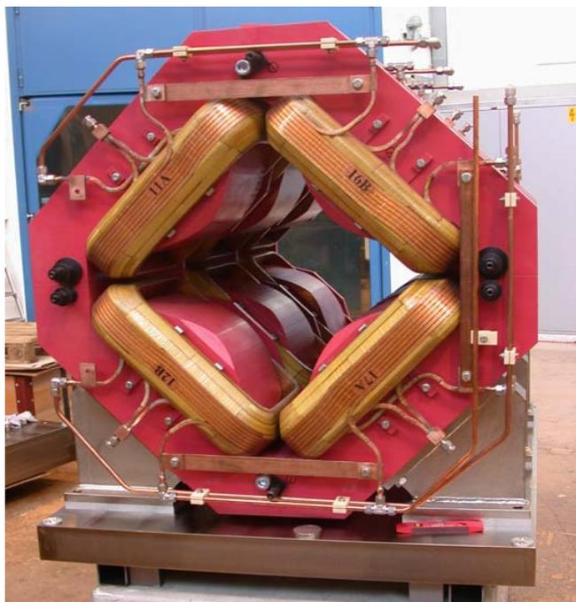
**Fig. 7:** The first triplet on its base plate during assembly. The mirror plates have not yet been mounted.
